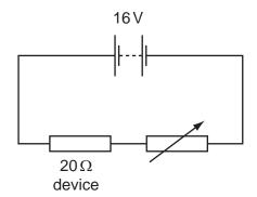
What is the resistance of the variable resistor when the power dissipated in the electrical device is 4.0 W?
