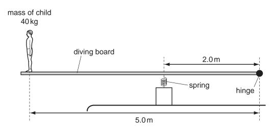
What is the extra compression of the spring caused by the child standing on the end of the board?
