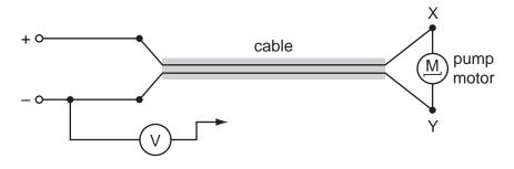
The motor does not work so, to find the fault, the negative terminal of a voltmeter is connected to the negative terminal of the power supply and its other end is connected in turn to terminals X and Y at the motor.
